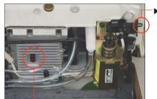
Maintenance Thanks to safety switch, during repair or maintenance work, the machine is not activated when its pedal is accidentally stepped on. Safety accidents are preventable.
