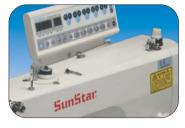
▶ Easy to Use Bobbin Winder The device to wind lower thread is installed on the top of the machine. The thread volume control and lower thread winding are much nare convenient.
