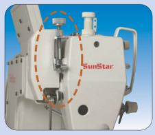
The delicate preser foot lifter is installed on the front side. It makes frequent adjustment of the height of presser foot much easier.
